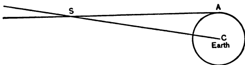
FIG. 45. — Horizontal parallax of a body at S . The circle represents the earth.
